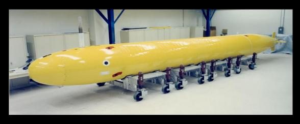
The first of two Draper-designed Unmanned Undersea Vehicles began at-sea testing for DARPA. These autonomous testbeds were designed around Draper's fault-tolerant processor and vehicle control architecture and were used to test mission packages.
